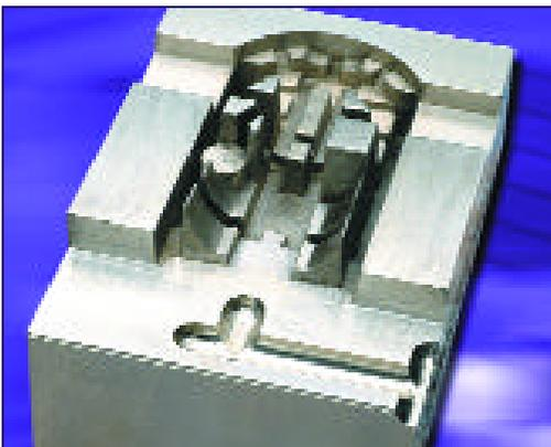
Mold insert using LaserForm ST-100 material
