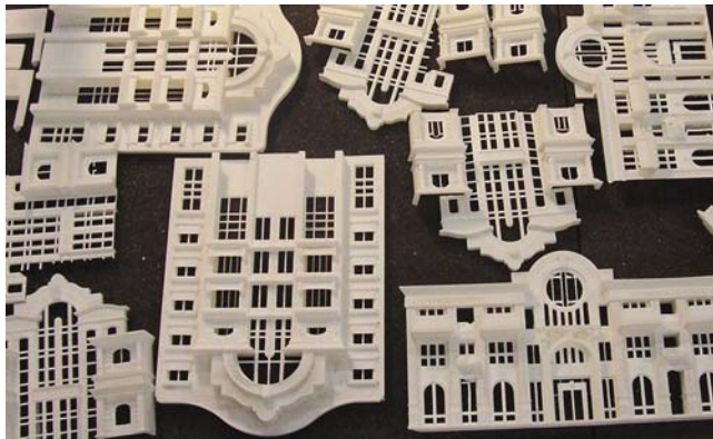
Each apartment building model in the Canal Residence West was made up of around 30 individual parts printed on the InVision® SR 3-D printer.
