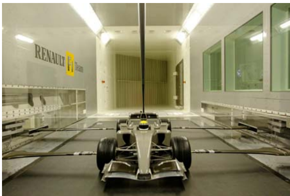
Parts produced in the ADM Centre are directly mounted to the wind tunnel model for testing.
