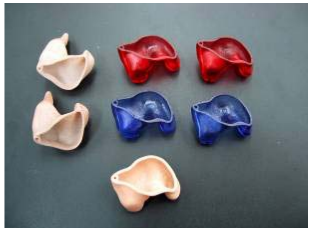
Red and Blue hearing aid shells are now produced in one single vat at the same time. No need to change vats to change material.
