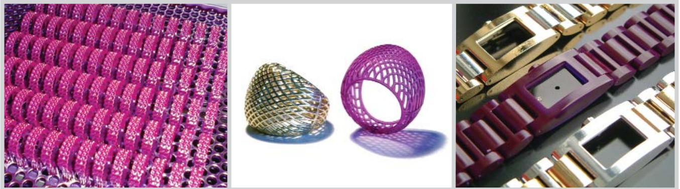
Left: Produce models, master patterns, design alternatives, or size variations in a single build. This platform of 90 rings was built in 16.2 hours, automatically. Right: Amethyst models (center) can be plated (top and bottom) or painted.
