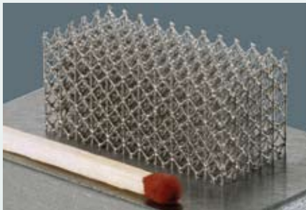
Ultra-light structure in aluminum.
