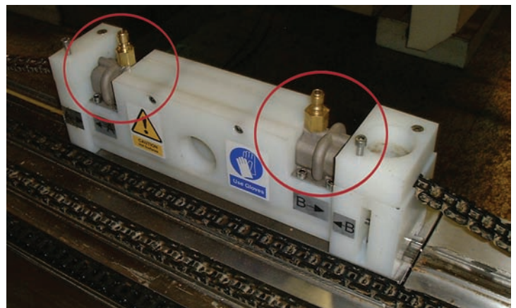
The new manifold (photo above) built on 3D Systems' SLM System for the conveyor cleaning system for a bakery replaced the old manifold (below), allowing the chain to be cleaned and eliminating the need for replacement every year.
