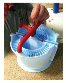
Full casting pattern of stator case.
