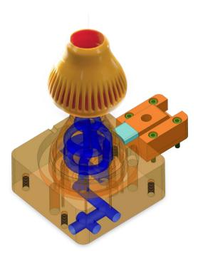
Complex conformal cooling channels created with the comprehensive mold design toolsets of Cimatron<sup>™</sup> led to a 14% reduction in cycle time and 16% reduction in overall costs.
