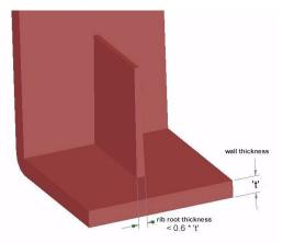
In some cases, using a glass-filled material will help avoid sink in geometries when adhering to the rule of thumb is impossible.
