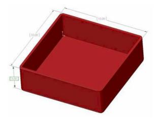
Size Limits for Rapid Injection Molding is 20" x 20" x 3"
