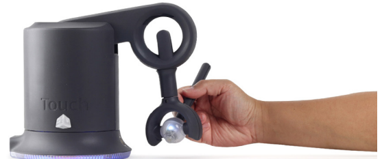
Using your wrist, rotate the stylus to the right.
