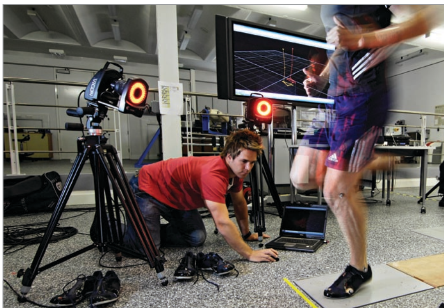
A researcher uses a 3D motion analyzer and force plate to measure the stiffness of soles being tested by athletes in a quest to bring more gold medals to UK Olympians.
