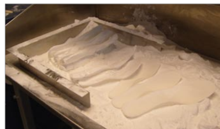
The spike soles were manufactured in a Vanguard selective laser sintering machine.
