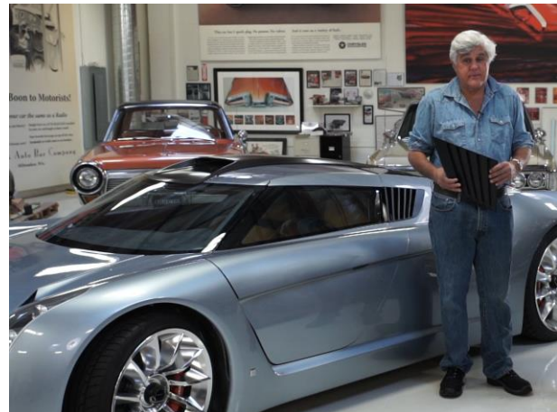
Jay Leno and his team used 3D design and manufacturing solutions from 3D Systems to replace and reproduce vents on the EcoJet concept car.
