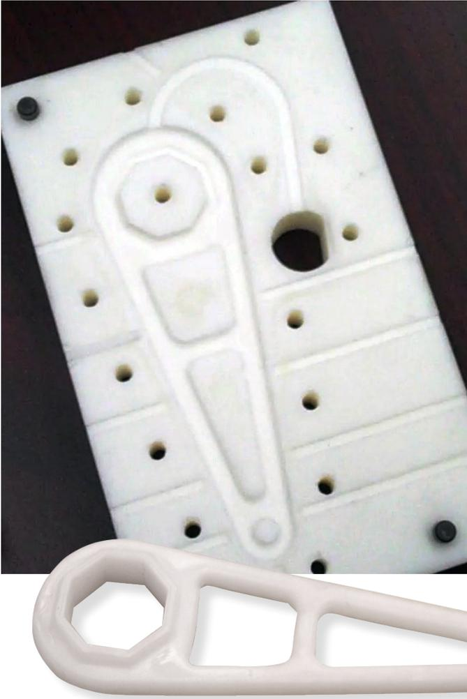
Thornton says that Teleflex has used the 3D-printed molds to produce more than a dozen different components from materials that include polycarbonate, ABS (acrylonitrile butadiene styrene) and LCP. He expects 3D printing to continue playing a major role in his company's experiments with new designs and materials.
