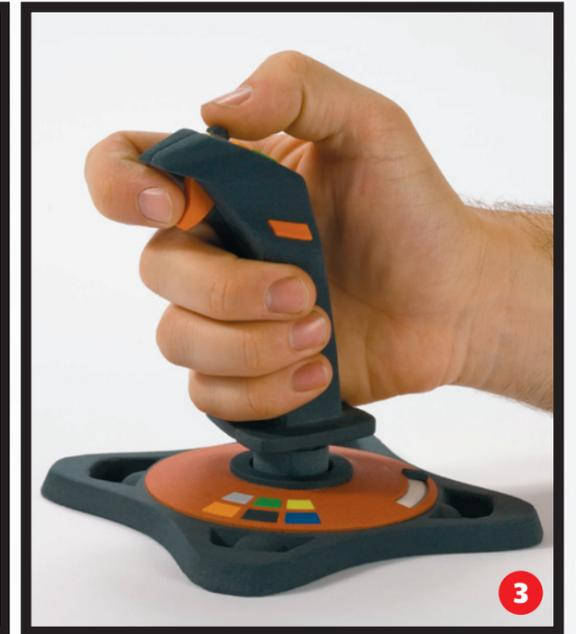
huge advantage: colour. By using separate colour binders, the system can print colour directly into each layer at its periphery where required, allowing full-colour, high-resolution models. So what's new for the 650? The answer is in three parts.
