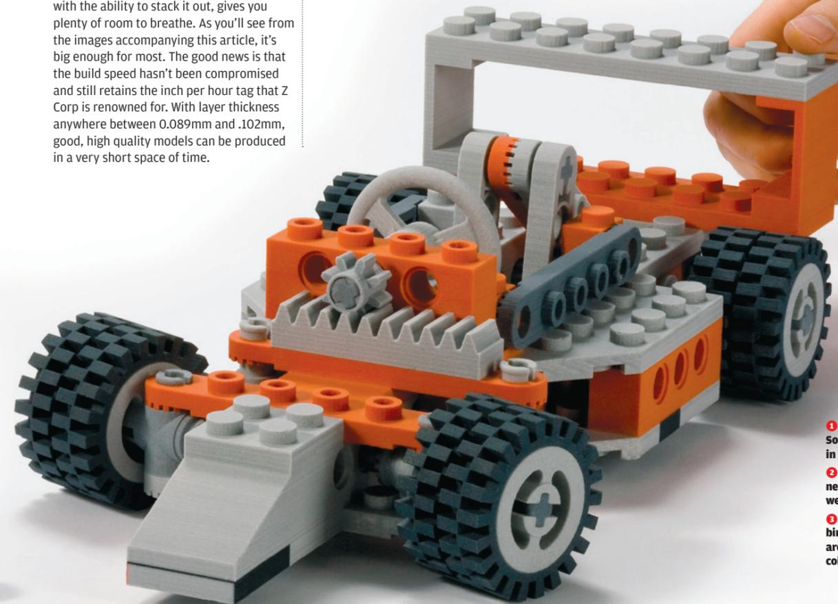
1 Modelled in SolidWorks, printed in one build
