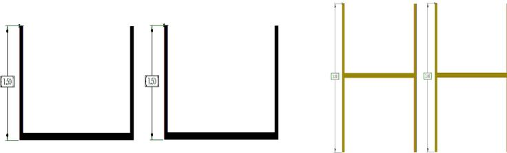
The Depth Limit is 1.5" for parts where the parting line is on the edge of the part, and 3" for parts where the parting line is central to the part.
