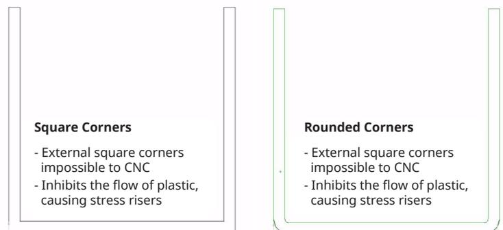
It is strongly advised that you ensure your design has rounded corners on every rib-to-wall or wall-to-wall intersection. This design consistency will result in a part with less internal stress—reducing the chance of warp, short shots, splay and flash regardless of which injection-molding process you use.
