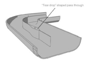
Always apply generous fillets to baffles to prevent side walls of ducts from splitting, especially if component will be exposed to pressure and/or cycling of temperature.
