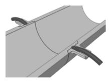
Above cross section shows glue (dark) getting sucked into radial cavity through access ports.
