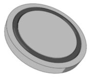
Negative Overhanging Draft to retain Elastomeric Gasket
