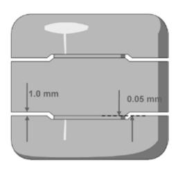
To solve this, one approach is to apply a form where the hinge rotates into a flush position. Generous tolerances in excess of 1mm can be applied in the disengaged state for building, while tolerances of approx 0.05mm will enable a flush intimate stable interaction in the engaged functional range of the rotation.
