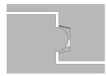
Allow 0.3mm+ clearance everywhere else. Note you also continue the pocket to punchout the side. This will have no effect on hinge functionality, however it will enable much quicker and complete powder removal.
