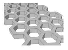
Also note that while you may cut down on the weight of the final part relative to a solid nongrid section, you will increase cleaning time and you will increase draw time on the systems, as the laser now outlines and fills in the feature rich cross-sections.
