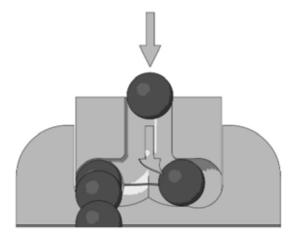
Once all the bearings have been dropped into the chase, a plug can be fixed to seal in the chase.
