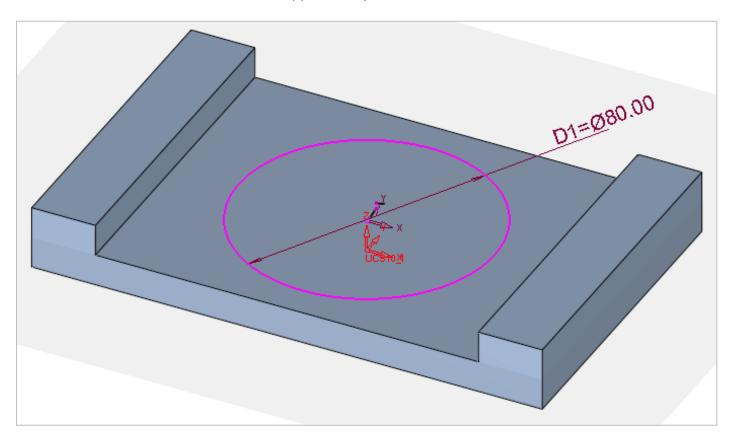
**14.** *Pick* the "Extrude" command , Set the parameters as shown in the picture, note to set it to "Add". After setting approve it by "OK" .
