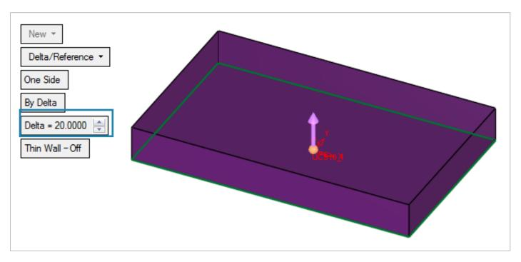
**8.** *Pick* the Sketcher Command and *pick* the top face of the box as the sketch plan. On that plan we will do the following:
