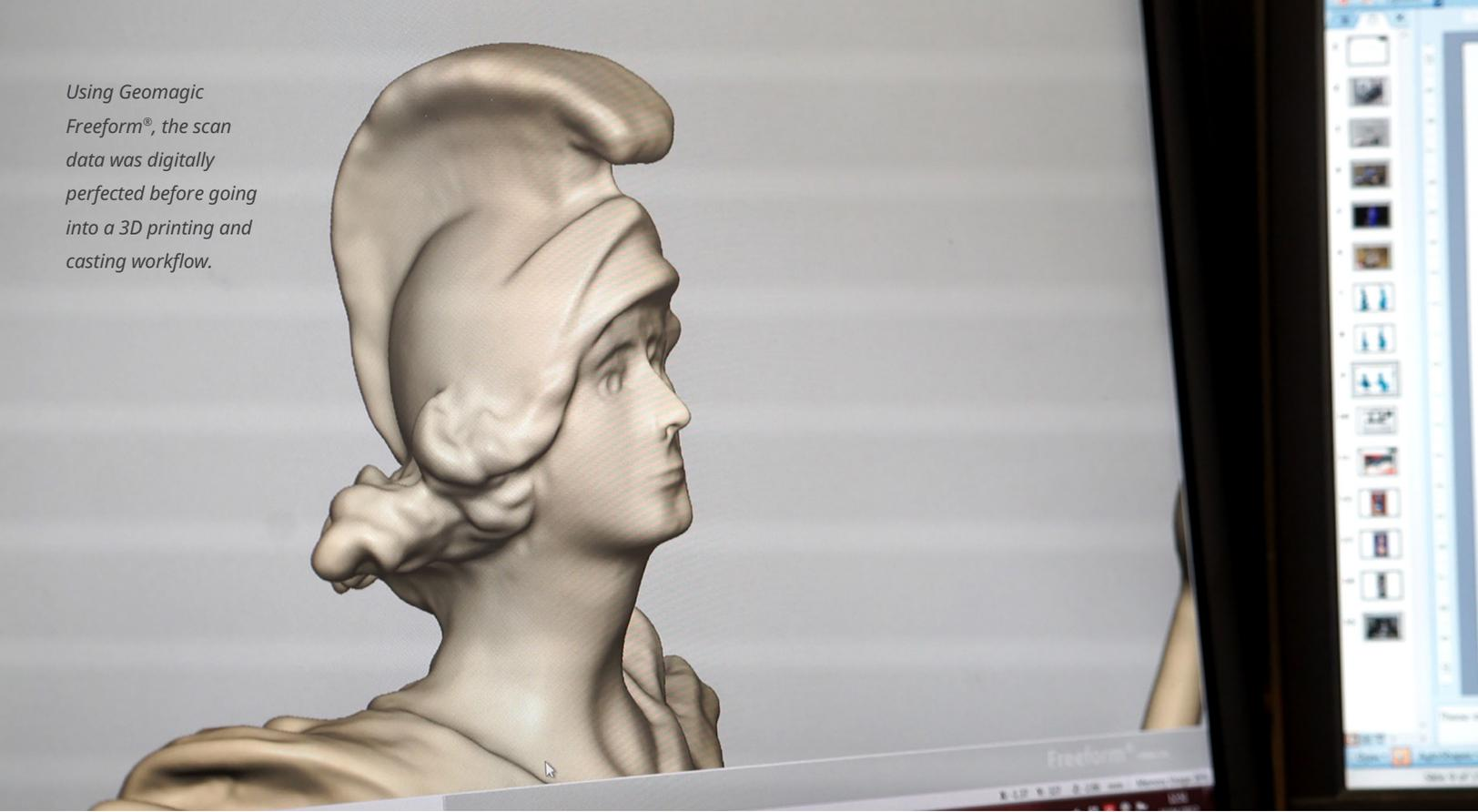
"Whenever we did something that didn't come out quite right, we pressed Control-Z to undo the move and redid it until we got it right," Carter said. The team designed the mounting hardware in SOLIDWORKS CAD system and exported STEP files which were imported into Freeform and subtracted from the Britannia model. Freeform was then used to reduce the model to half its original size.
