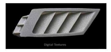
Initial cost of tooling for traditional injection molding created in-house was \$4,850 versus no tooling costs for digital molding based on 3D Systems Figure 4 technology. The volume justification for choosing digital molding over conventional injection molding in this case is up to 700 units.
