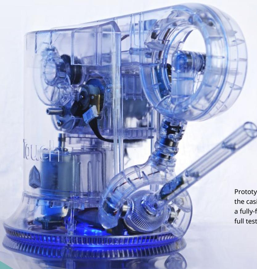
Prototype Touch haptic device with the casing printed in ClearVue allows a fully-functional working design for full testing and assembly checks
