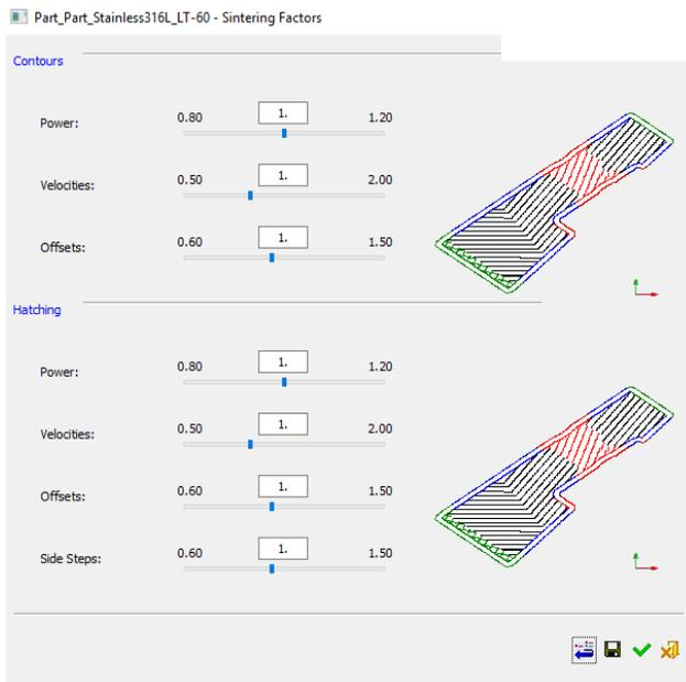
This dialog enable to control global Laser Power and Velocity & Offset values for both Contours and Hatching, and also the Side Steps for Hatching.
