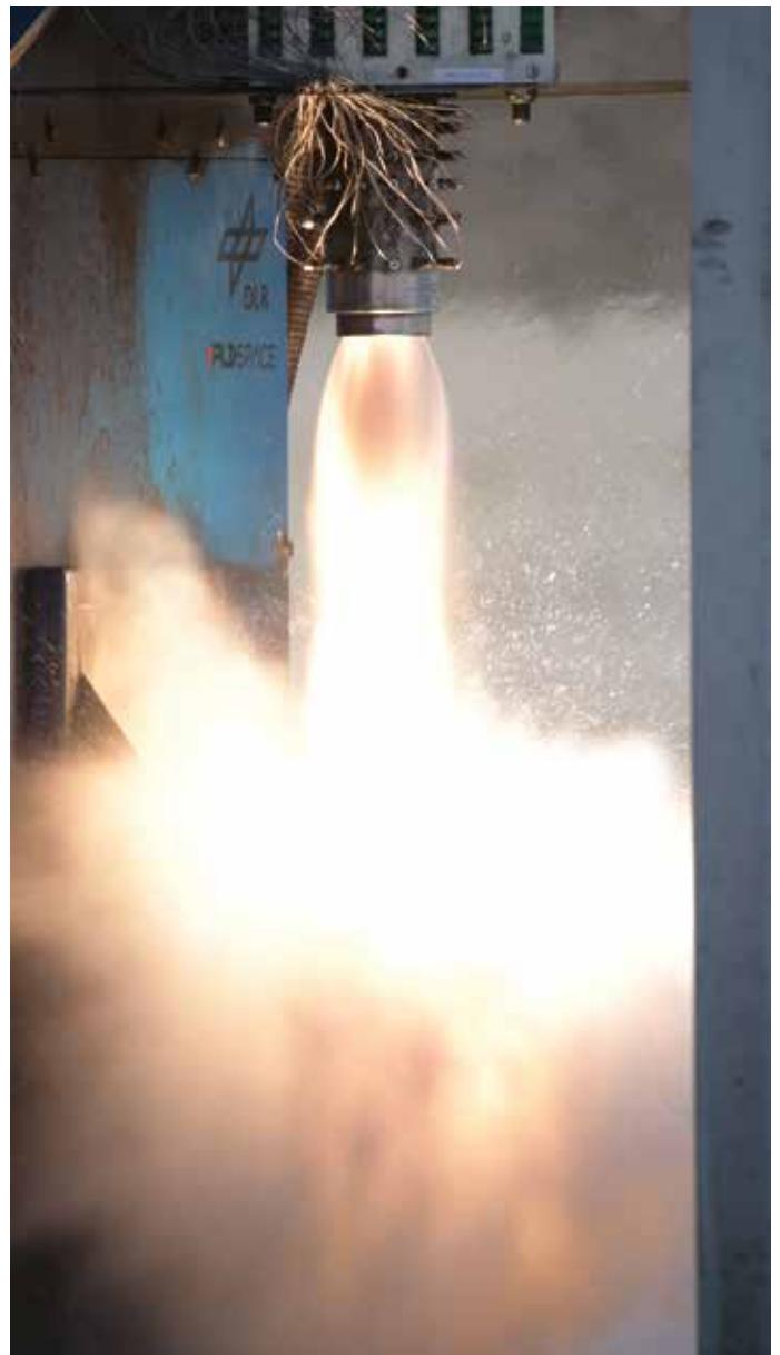
Hot-fire testing of the 3D printed injector head showed good mixing and combustion efficiencies.
