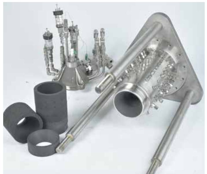
Setup of LOX/kerosene rocket engine with 3D printed injector (partner: 3D Systems) and ceramic combustion chamber
