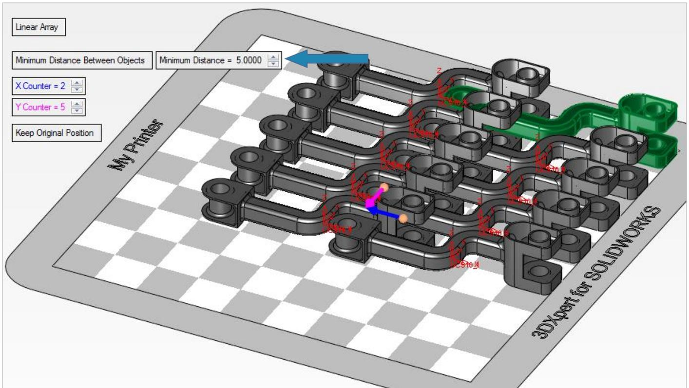
Note that in this mode of **Minimum Distance** the X&Y Delta are not displayed and that the systems ensures that the parts do not touch each other.
