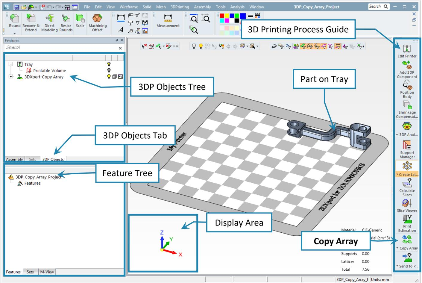
3. From the 3D Printing Process Guide access **Copy Array**
