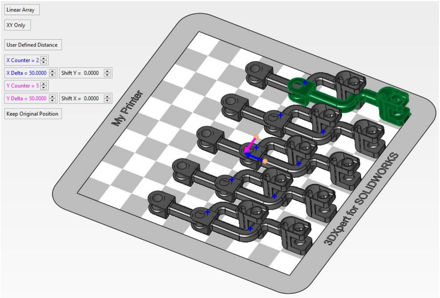
7. It is possible to copy array on **XY only** or also on Z direction. Change the parameter XY Only to **XY & Z**. In this case, a 3D array is created in the X, Y and also Z direction.
