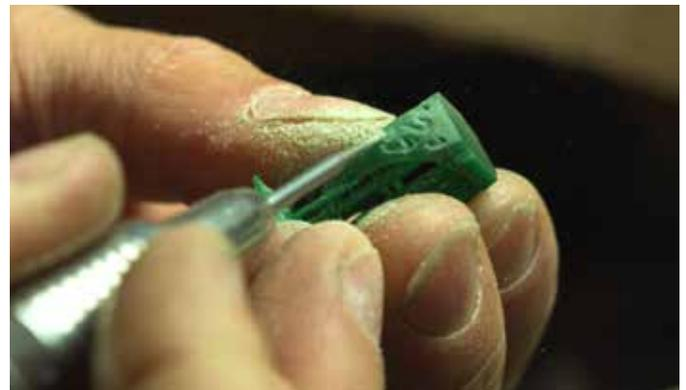
*The ability to adjust 3D printed designs using bench techniques helps Artforge Studio accommodate changes requested by its customers.*
