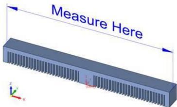
Avoid measuring near the corners of the part, as corners are further deflected.
