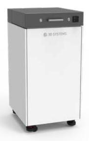
Equipped with 16 UV light bulbs placed inside of the four walls, the Figure 4 UV Cure Unit 350 achieves highly efficient and uniform curing. The interior allows you to cure parts on the build platform or place parts on multiple shelves to cure more parts at once, and is optimized for Figure 4 Modular parts at the maximum build height of 346 mm.
