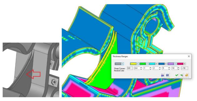
3DXpert's has all the modeling tool to modify the part accordingly, such as to offset faces in order to thicken the ribs or move the ribs further apart.
