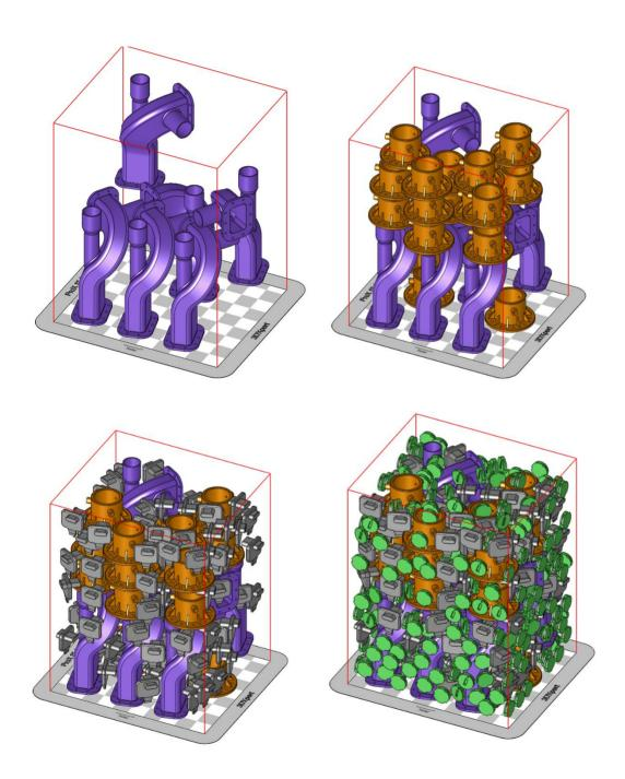
In this example, the largest part, a manifold (purple) is placed 6 times, the pipe bracket (orange) 19 times, the key (grey) 107 times and the cover (green) is placed 432 times.
