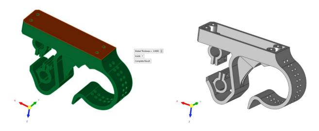
You can also can add drain (or escape) holes so that the unsintered powder can be easily removed after printing.
