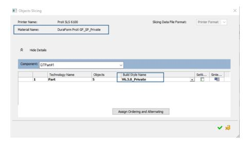
It is not possible to assign different Technologies (build styles) to different objects of a single part (component).
