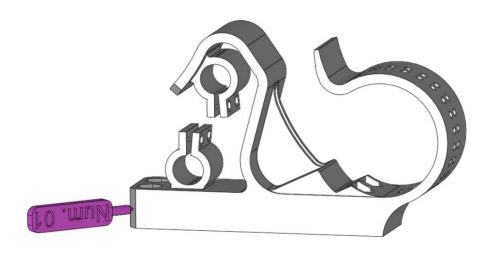
A detachable label, connected to the part, to be removed after printing.
