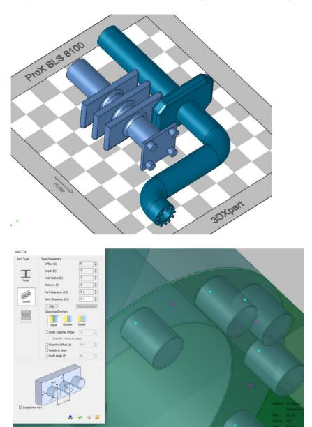
The part can be split along any plane or along a contour. There is full control over the connecting dowel's parameters (such as radius, depth, chamfering and clearance). Here are some examples for Joint Cut parameters:
