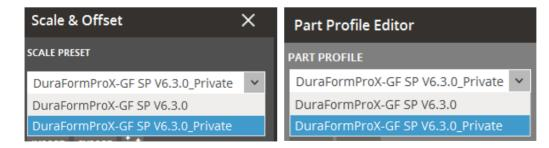
The result is that any 3DXpert build style for ProX SLS 6100 is a combination of Scale & Offset and Part Profile.
