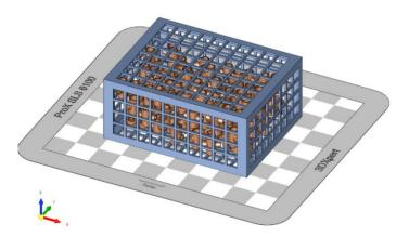
Sinter Box includes various options, such as creating a totally sealed cage or a perforated cage, setting for the thickness of the cage and margins from the tray boundaries, adding text to the cage and more.
