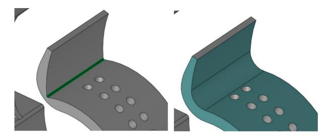
With SLS it is common also to hollow the part, in order to avoid deformation during the printing process.
