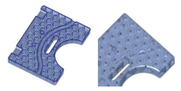
The above images show an internal honeycomb Infill structure. Such walls inside the volume also increase the stiffness of the component. Hollowing a part this way may also reduce warping.
