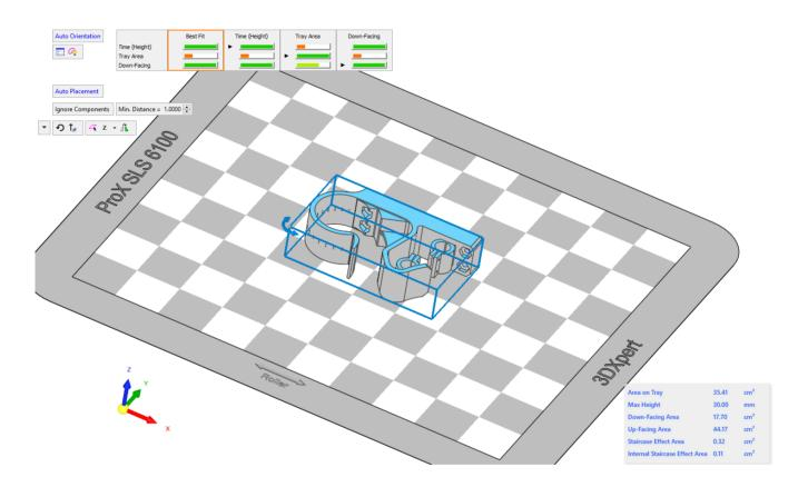
As mentioned above, the design for SLS must consider this technology for wall thickness, holes size, channels, engraving and so on.
