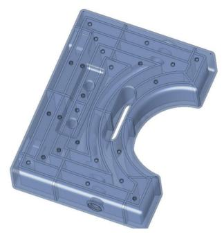
Conformal Infill - Notice the way that the walls follows the different areas of the volume.
