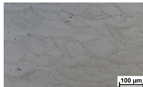
Microstructure without heat treatment (NHT)
