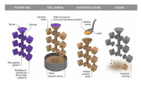
3D printed patterns are burned out into the lost wax or shell investment casting process
