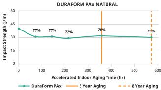
OUTDOOR STABILITY: Tested per ASTM G154 standard method.
