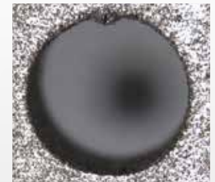
Example of a horizontally built hole
