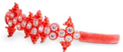
Print crisp details on small features and micro-pave settings. Consistently achieve the highest level of precision and repeatability by adopting a digital foundry workflow for jewelry manufacturing.
