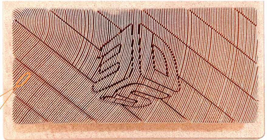
Part: Heat exchanger Bounding box: 420x200x100 mm Layer Thickness: 40 µm Print time: 27h
