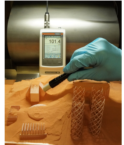
Electrical conductivity measurement after printing using the Electromagnetic (Eddy Current) method
