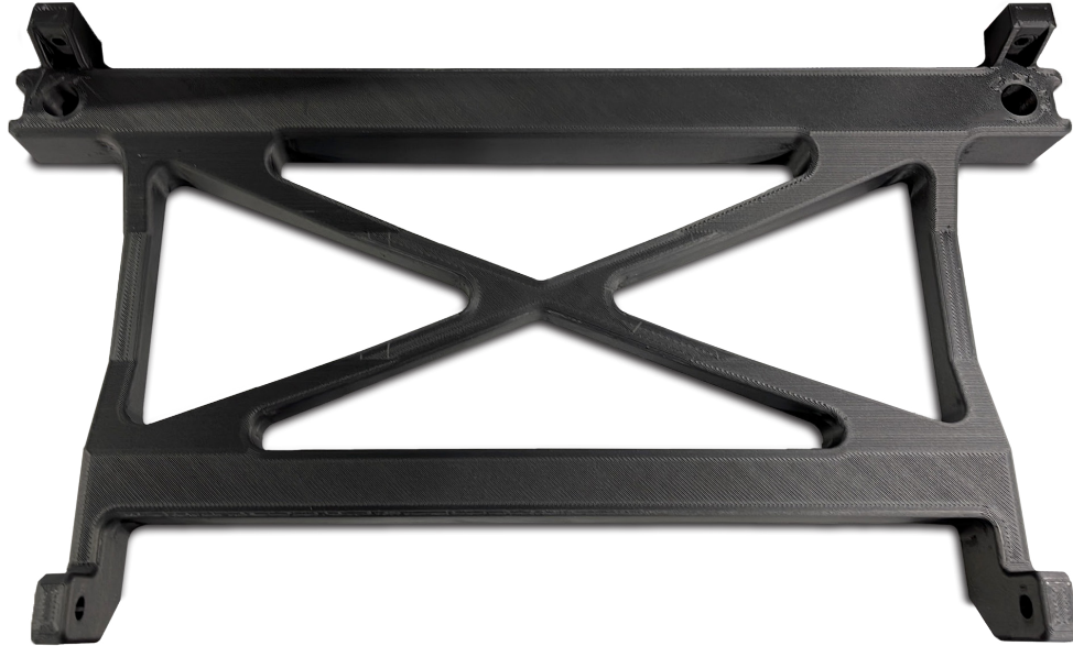
Fig 13 – Printed quality gage ready for machining
