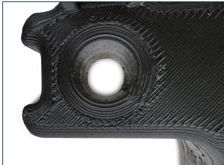
Fig 12 – Locator pin hole shown in Fig 11, as-printed
