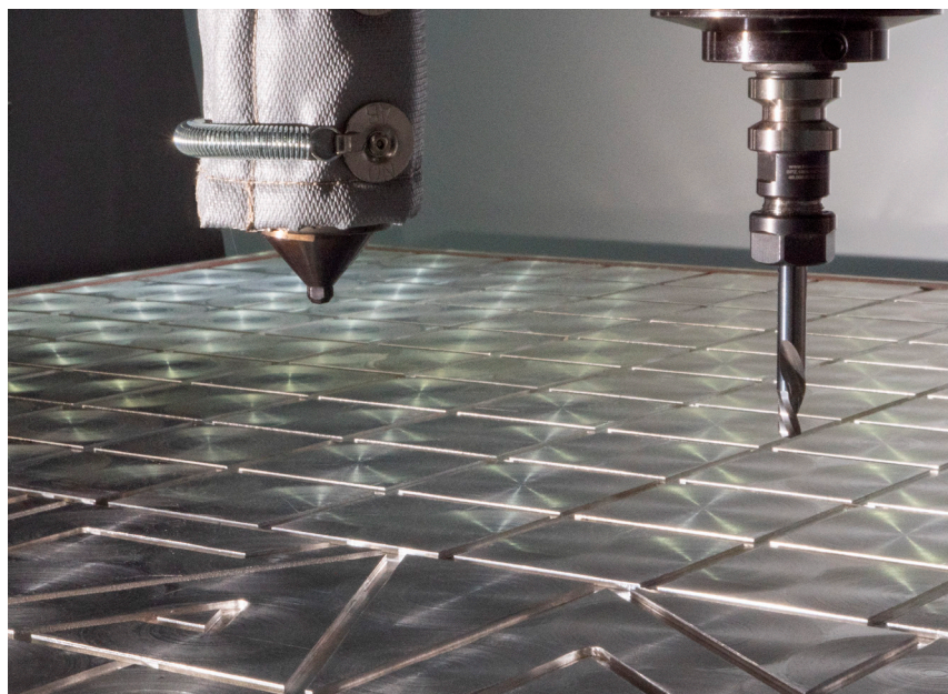
Fig 16 – Pellet Extruder and Milling Spindle Toolheads on EXT 1070 Titan Pellet 3D Printer
