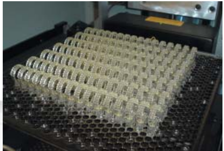
In high resolution mode it builds 44 rings (even different ones) at a size of 6 mm x 22,5 mm x 21.3 mm in only 10 hours
